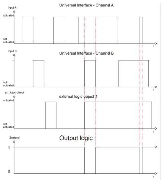
In the figure above, only when three inputs are 1, And operation result of the is 1, the output of the reverse is 0, And the other time output is 1.
