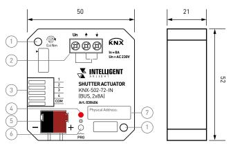
M3 screw fixed installation hole position \*2, suitable for non-concealed box type fixation
