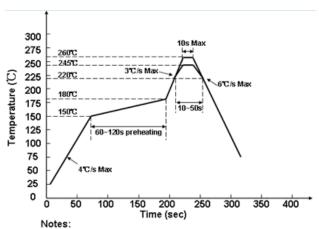
We recommend the soldering temperature 245 $\pm$ 5 $^{\circ}$ C; The maximum temperature should be limited to 260  $^{\circ}$ C.
